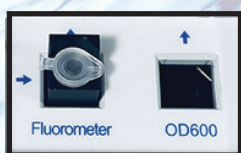
Fluorometer & Cuvette OD600 ports
