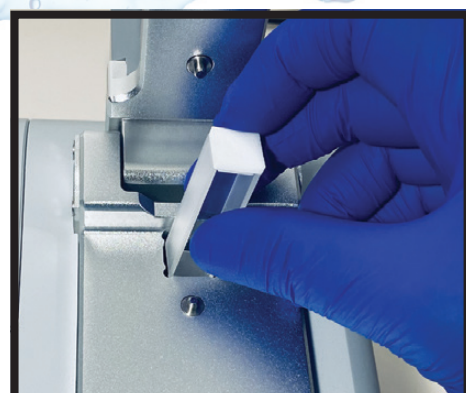
Cuvette port for OD600 readings
